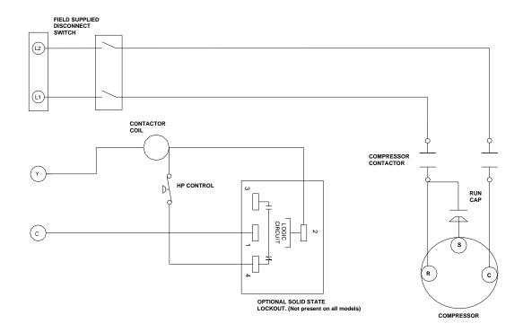
This diagram is provided as reference only. Wiring may differ depending on unit. Always refer to correct wiring diagram locate on inside cover of electrical panel Optional items that may be present:
